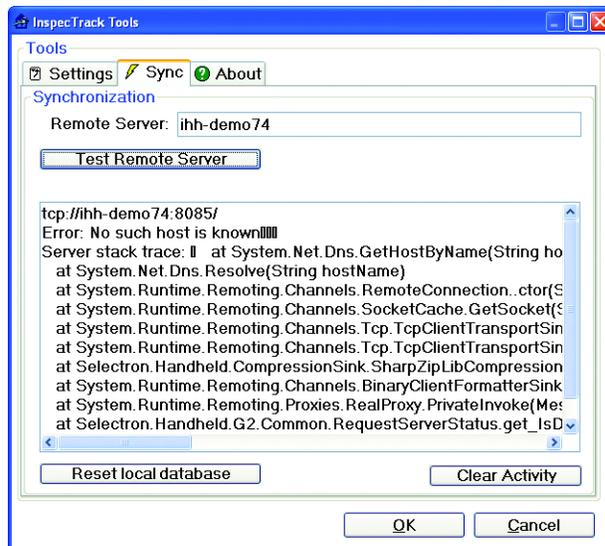
Figure E-8 Sync tab displaying no connection to remote server message
