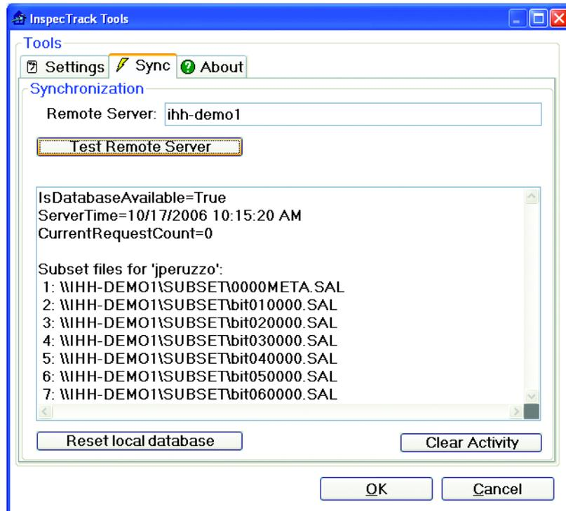
Figure 6-6 Sync tab showing successful connection to remote server
